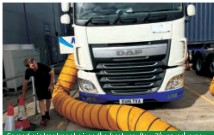
Forced air treatment gives the best results with no adverse effects on the vehicle's sensitive electronics
