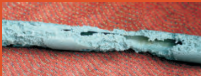
First the mice gnawed the pipe insulation, presumably for bedding, then...
