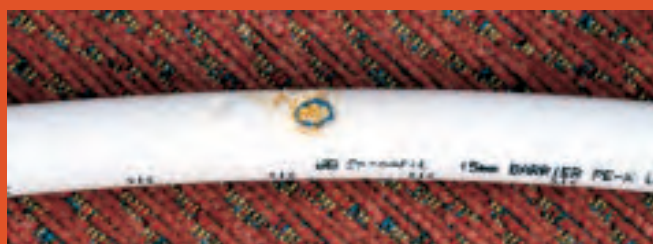
...having got through to the water pipe, they made a hole that caused a leak
